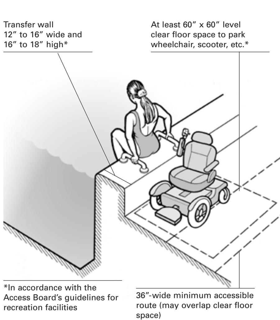
**Figure 16. Transfer System (lift or transfer system
